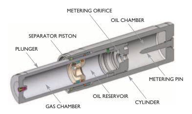
The illustration shows the robust construction of the Oleo hydraulic unit. Under impact the plunger is forced into the cylinder displacing oil through the orifice, moving the separator piston and compressing the gas. The compressed gas acts on the oil through the separator piston to give recoil force to re-extend the unit after impact. The energy absorbed and dissipated is dependent on the closure velocity.
