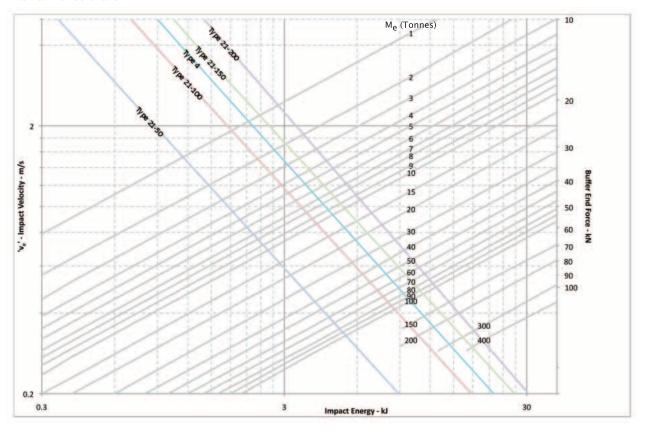
Before using the chart, it is necessary to know the impact Mass ' $M_{e'}$ ' and the impact velocity ' $v_{e'}$ ' of the moving machine. On very wide track machines such as travelling cranes, the mass on the rail can vary considerably due to asymmetric loading, or the position of the trolley. In these cases the maximum mass on the rail MUST BE used and each side of the bridge dealt with separately.
