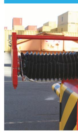
The Type 70 buffer is a long stroke 700kN buffer available with 500mm and 600mm stroke. These are typically used on dockside cranes and in steel mills. The Type 70 buffers are also used on mining applications as they can be used vertically. They have also been used as end stops for funicular railways as they have the ability to be set at an angle.
