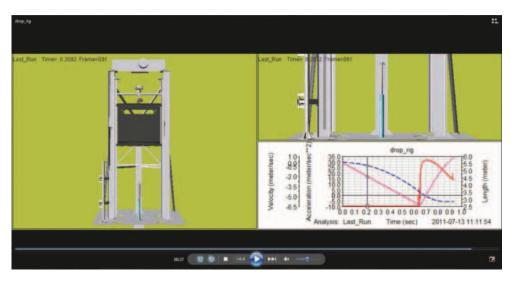
Oleo provide elevator impact simulation to validate test results
