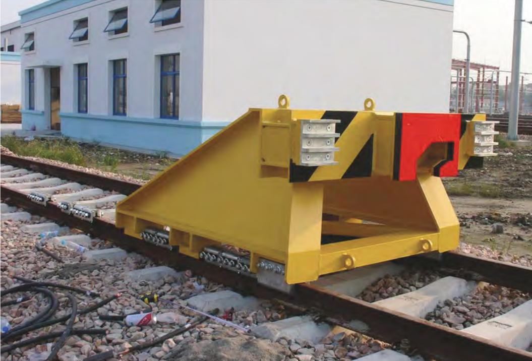
Train mass: 408 tonnes Impacting speed 25km/h fitted with seventeen pairs of friction shoes with an installation length of 15m.
