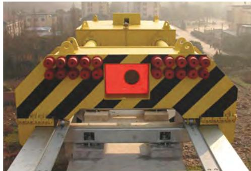
Typically used on low speed test lines – designed for centre and side impact. Fixed end stops incorporating Oleo hydraulic units (two Oleo Type 718 – Recoverable stroke 1800mm). Installation length: 5.5m, Impact capacity 2016kj.
