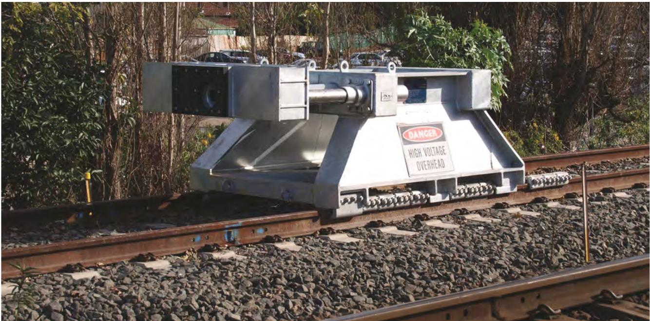
Typically used for main lines – designed for centre impact only. Sliding friction end stop with nine pairs of friction shoes and one pair of anti climber shoes at the front. Incorporating Oleo hydraulic units (two Oleo Type 9 – Recoverable stroke 400mm). Train mass: 535 tonnes, Impacting speed: 25 km/h, Installation length: 16 metres, Impact capacity: 448 kJ.
