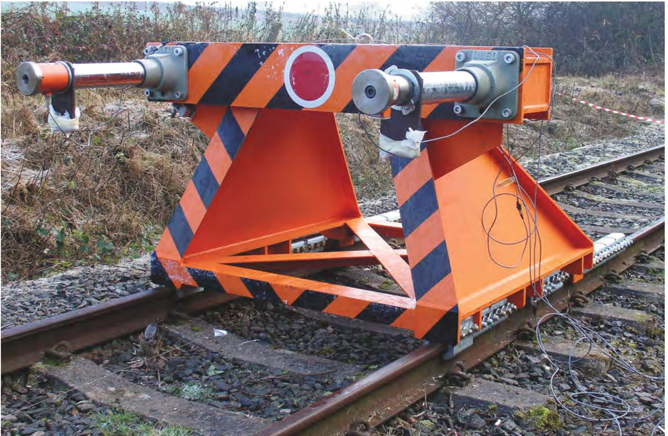
Typically used on European main lines (freight) – designed for side impact only. Sliding friction end stop (eight friction shoes) incorporating Oleo hydraulic units (two Oleo Type 9 – Recoverable stroke 400mm). Train mass: 220 tonnes, Impacting speed: 25 km/h, Installation length: 25 metres, Impact capacity: 448kj.
