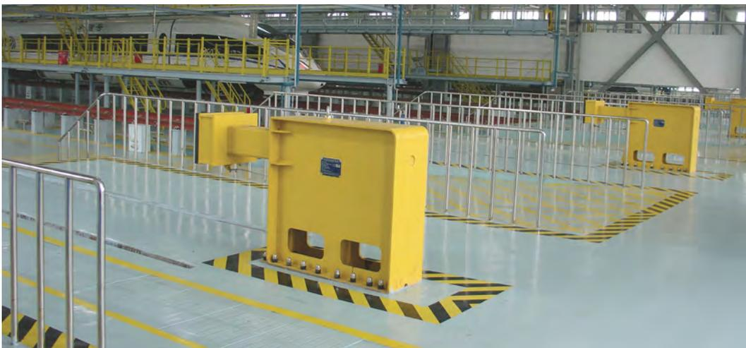
Typically used on depot/maintenance workshop – designed for centre impact only. Fixed end stop incorporating Oleo hydraulic unit (single Oleo Type 76 – Recoverable stroke 600mm). Installation length: 2.7metres, Impact capacity 336kj.
