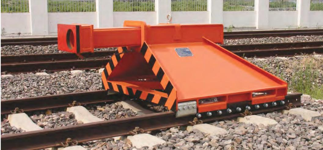
Typically used on 'end of line' – designed for centre impact only. Fixed end stop incorporating Oleo hydraulic units (one Oleo Type 76 – Recoverable stroke 600mm). Train mass: 300 tonnes, Impacting speed: 5km/h, Installation length: 2.8metres, Impact capacity: 336kj.
